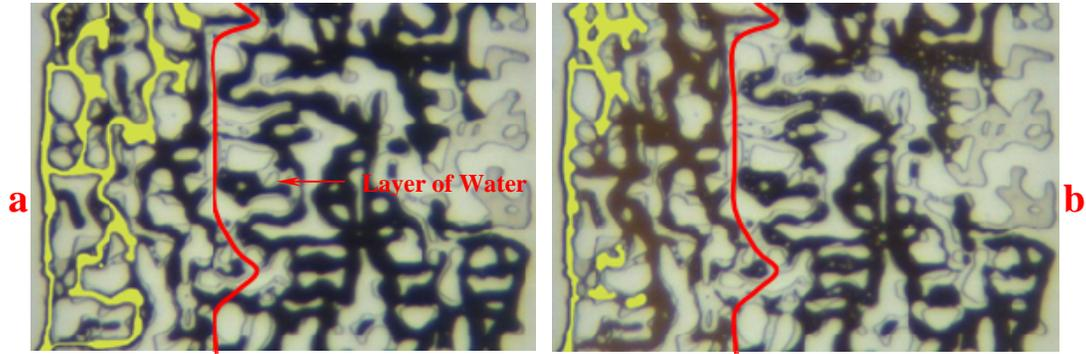
Figure 5: Crude oil dilution in the selected section of the micromodel during the first period of CO<sub>2</sub> injection after a) a few hours, and b) 2 days of CO<sub>2</sub> injection.
