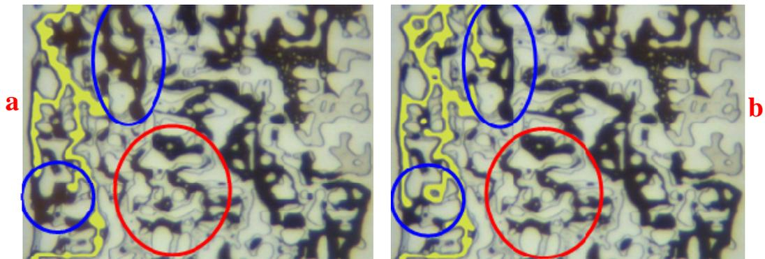
Figure 7: Crude oil colour change in the second period of CO<sub>2</sub> injection after a) breakthrough of CO<sub>2</sub> and, b) 24 hours of CO<sub>2</sub> injection. The areas which have been specified with the blue circles were in direct contact with CO<sub>2</sub> and became darker after the second period of CO<sub>2</sub> injection and the area in the red circle is example of the part of the oil which was not in direct contact with CO<sub>2</sub> and has retained its lighter colour.
