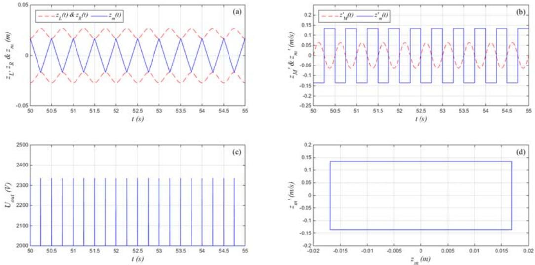
Figure 2. (a) Displacements and (b) velocities of the outer structure and the ball, (c) output voltage versus time for  $\beta=0^\circ$ ,  $r = 1$ ,  $A=0.1$  N and  $f_0 = 2$  Hz under saw-tooth initial conditions, and (d) the ball's phase trajectory.
