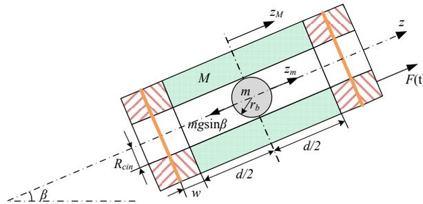
Figure 1. Sketch of the proposed DE-based dynamic vibro-impact system
