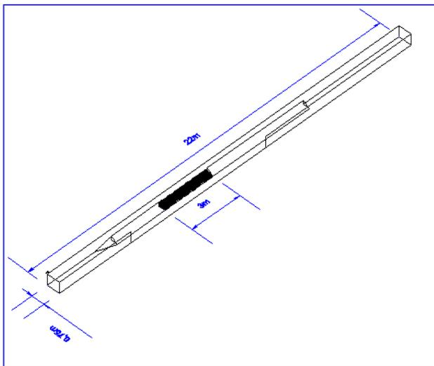
Fig. 2: Schematic view of Geobag setup in flume
