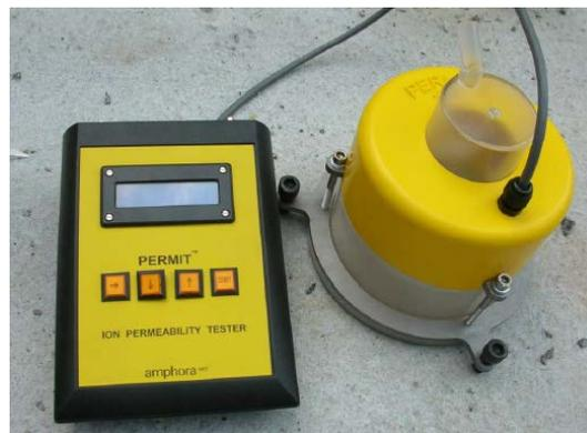
**Figure 4:** The PERMIT ion migration test apparatus
