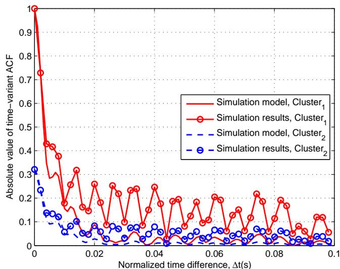
Fig. 7. The comparison of time-variant ACFs of simulation model and simulation results ( $f_c = 58$  GHz,  $D_{pn,m_n}^T(t_0) = 50$  m,  $D_{qn,m_n}^R(t_0) = 100$  m,  $\lambda_G = 80$ /m,  $\lambda_R = 4$ /m,  $v_{n,A} = 30$  m/s,  $v_{n,Z} = 30$  m/s,  $v_R = 100$  m/s).
