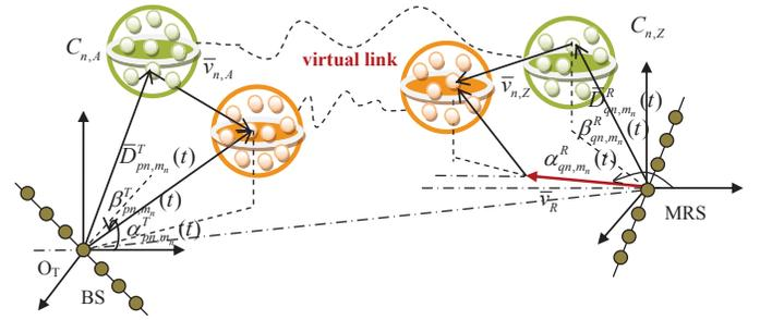
Fig. 2. A 3D non-stationary twin-cluster HST channel model.
