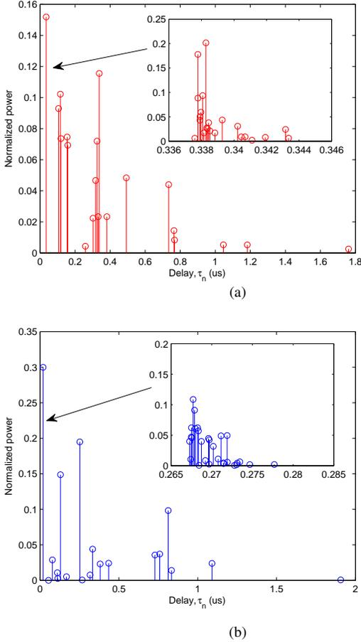
Fig. 5. The delay PSDs of the non-stationary HST simulation channel model at (a)  $t = 2$  s and (b)  $t = 4$  s ( $D_{pn,m_n}^T(t_0) = 50$  m,  $D_{qn,m_n}^R(t_0) = 100$  m,  $\lambda_G = 80$ /m,  $\lambda_R = 4$ /m,  $v_{n,A} = 30$  m/s,  $v_{n,Z} = 30$  m/s,  $v_R = 100$  m/s).
