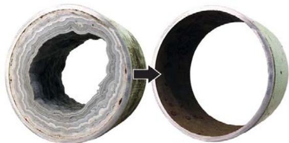
Figure 1 Pipe with scale deposits on the left and after scale removal on the right and [5]
