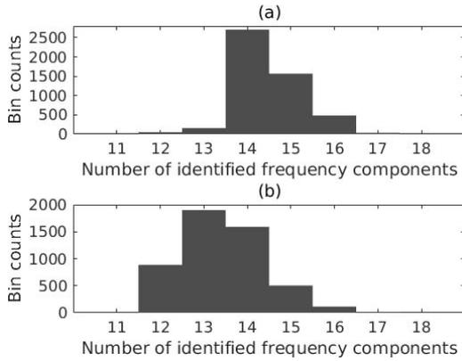
Fig. 2. Histograms showing the number of detected frequency components using 5000 rjMCMC realizations for (a) the original MB signal (1<sup>st</sup> round of signal reconstruction), and (b) the synthetic MB signal (2<sup>nd</sup> round of reconstruction).
