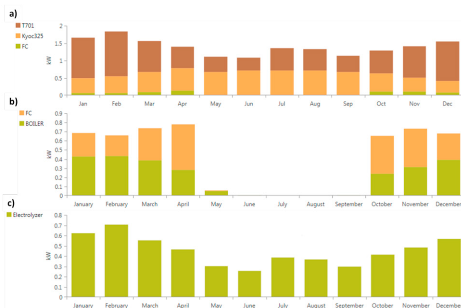
Figure 2: Monthly average a) electricity generation, b) heat generation and c) electrolyzer operation for hydrogen production from the hybrid system.
