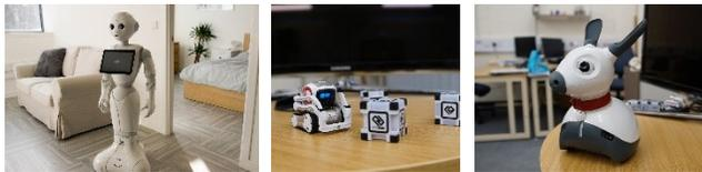
**Figure 1 Social robots demonstrated during Phase 2. Left: Pepper robot demonstrating upper limb rehabilitation exercises; Centre: Cozmo lifting and carrying its cubes; Right: MiRo acting as a social pet.**
