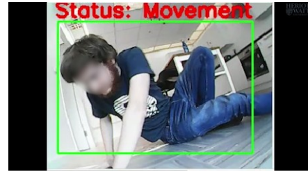
Figure 3 MiRo using computer vision algorithms to detect movement while a person is trying to get up. A green square is drawn around the area movement is detected.
