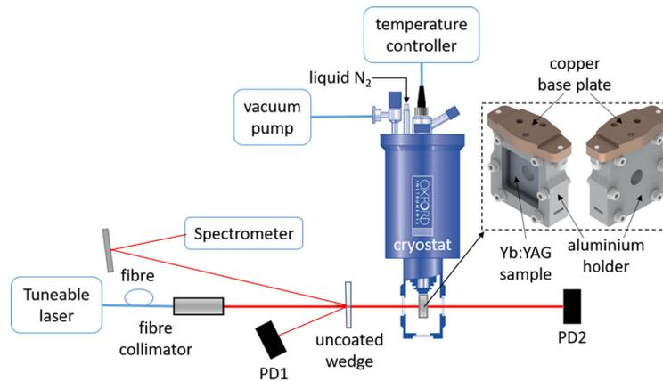
**Fig. 1.** Experimental setup used to characterise absorption at the ZPL of Yb:YAG (PD1, PD2 = photo-detectors). The insert shows frontal and rear views of the holder in which the Yb:YAG sample is mounted.
