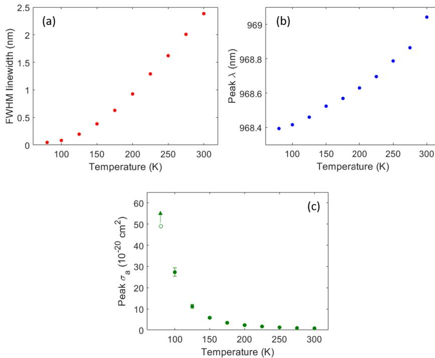
**Fig. 5.** ZPL characteristics between 80 K and 300 K: FWHM linewidth (a), peak wavelength (b) and peak absorption cross-section (c). The data point at 80 K represents a lower limit to the actual value of the absorption cross-section.
