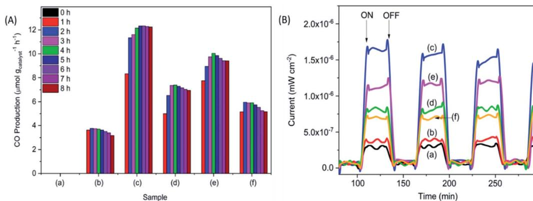
Fig. 3 CO production (A) and photocurrent (B) obtained from for the pristine P25 (a) P25-C (b) P25-NO (c) P25-NC (d) P25-KO (e) and P25-KC (f) under UV irradiation.
