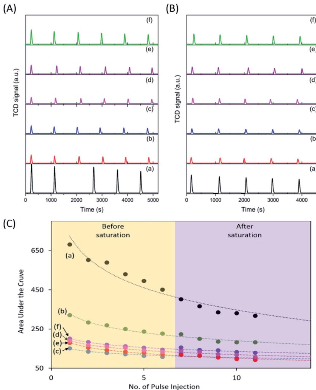
Fig. 2 Pulse injection of CO<sub>2</sub> performed on TPD before (A) and after (B) CO<sub>2</sub> equilibrated for 24 h, and the integrated area under the curve (C) for pristine P25 (a) P25-C (b) P25-NO (c) P25-NC (d) P25-KO (e) and P25-KC (f) under UV irradiation.
