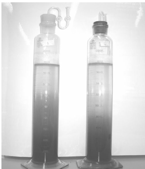
Figure 1. Two-liter cylinders used for the fermentations.
