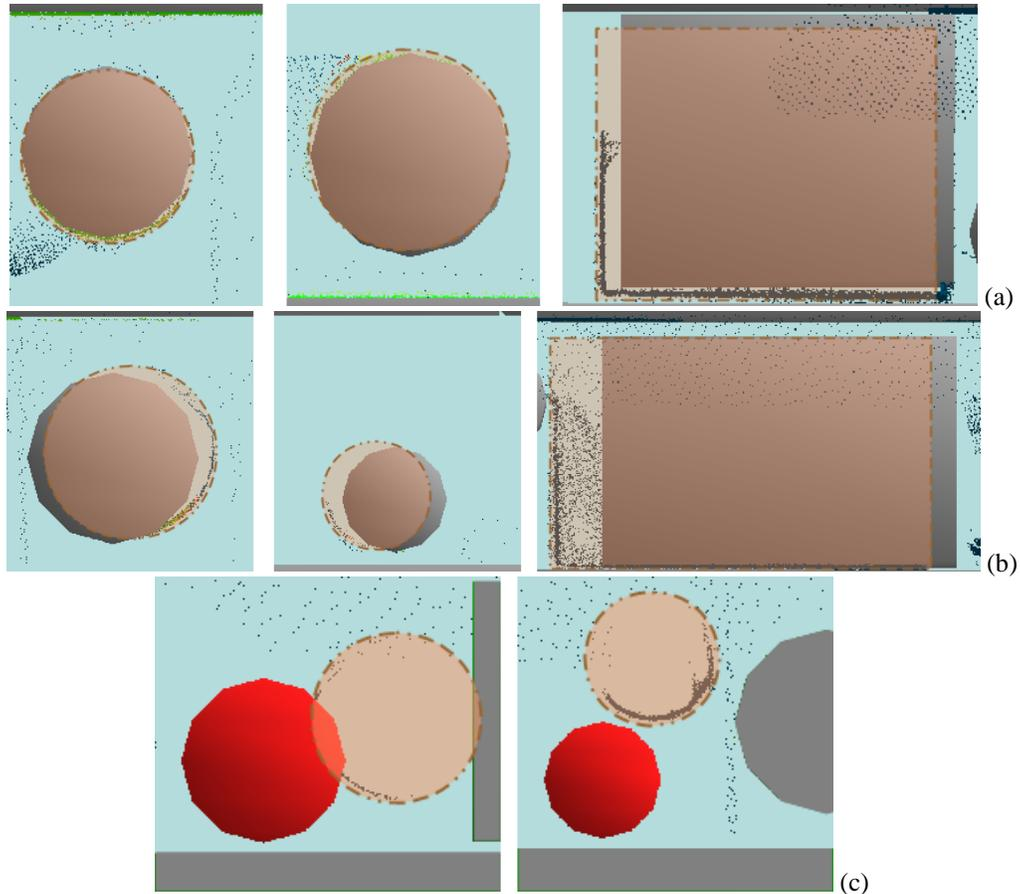
Figure 3: Correlation between level of confidence,  $\%_{\text{confidence}}$ , and deviation between as-built and as-planned poses of elements. The actual pose of each element (in the point cloud) is highlighted in transparent orange. Top row: Elements recognized with high level of confidence; Middle row: Elements recognized with medium-low level of confidence; Bottom row: Elements not recognized (false negatives).
