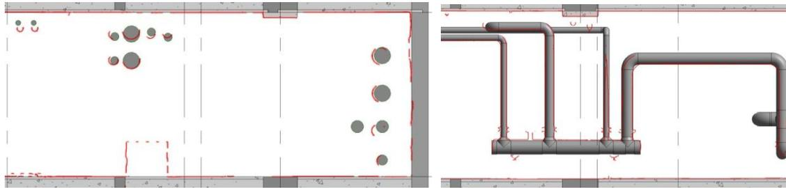
Figure 6: Two vertical cross-sections visualizing the comparison between the scanned data and 3D model for the 2<sup>nd</sup> basement.
