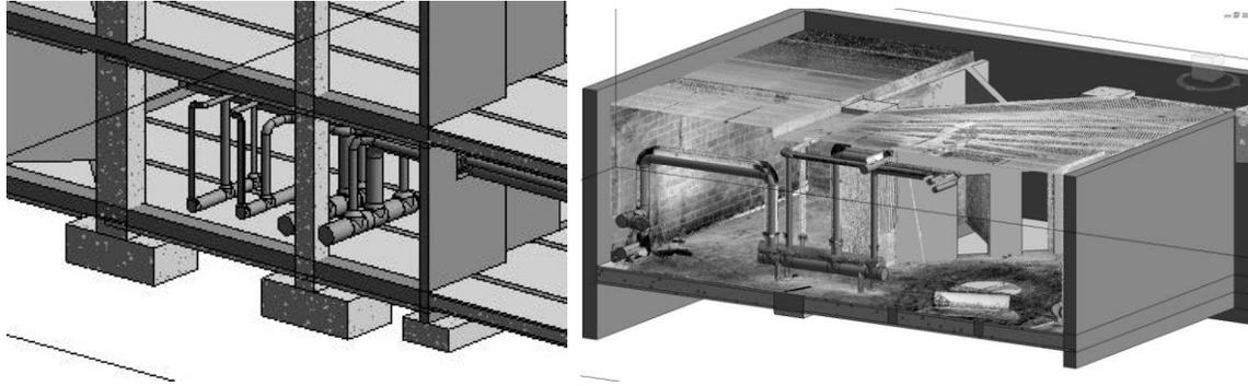
Figure 4: The 3D model (left) and the scans (right) for the service area in the 2<sup>nd</sup> basement.
