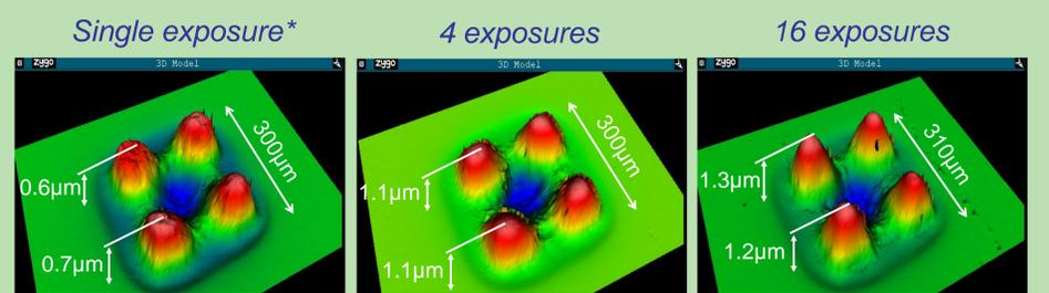
\* Single exposure = 13.33ms train of laser pulses at a 400kHz pulse rep-rate
