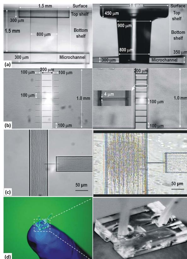
**Fig. 2** (a–c) Optical micrographs showing the components of the device before etching (left) and after etching (right) with HF at 13.3% (v/v) dilution for 4.5 h. (a) The inlet system viewed side-on. (b) Top view of the constriction array. (c) Top view of the T-junction. (d) The device on a fingertip with a magnified view shown alongside.
