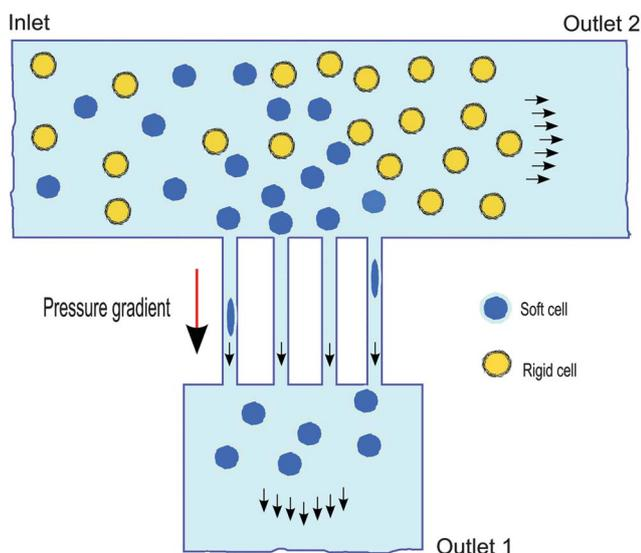
**Fig. 1** Schematic showing the working mechanism of the device. A pressure gradient applied between the two microchannels allows the relatively softer cells to squeeze through the constrictions to be collected at outlet 1.
