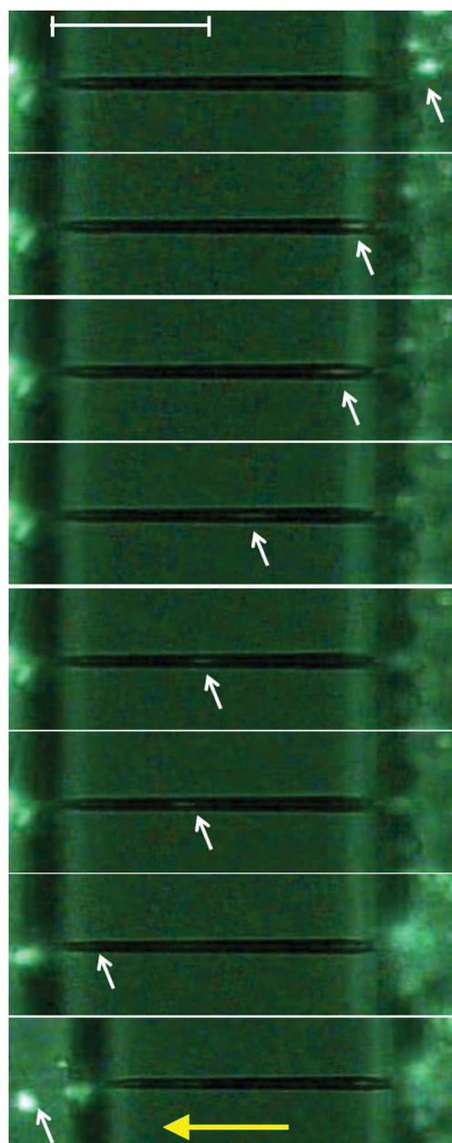
**Fig. 6** Fluorescence images showing the deformation of a single cell as it travels through the constriction in the multi-constriction device. The scale bar represents  $100 \mu\text{m}$ . The white arrows show the position of the cells. The yellow arrow indicates flow direction.
