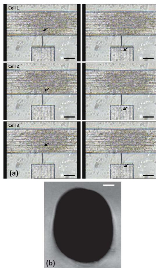
**Fig. 3** Optical micrographs of the single constriction T-junction device. (a) The HL60 cells can be clearly seen after they pass through the constriction (see supplementary material). Scale bar - 50  $\mu\text{m}$  (b) Cross-sectional view of a constriction. Scale bar represents 1  $\mu\text{m}$ .
