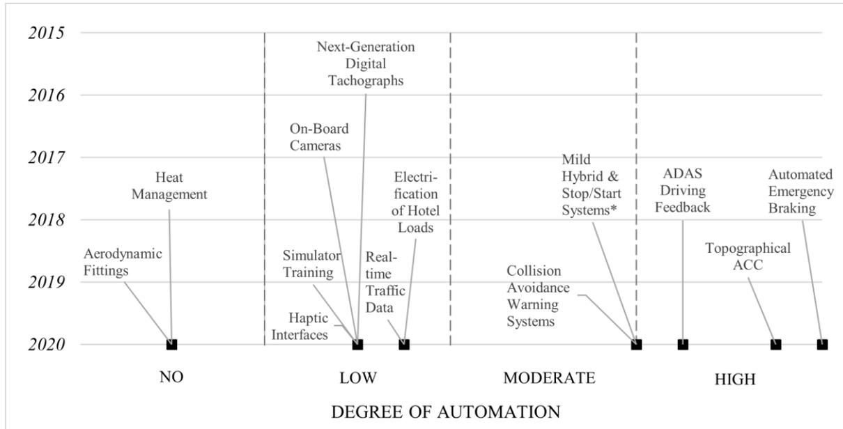
Figure 1: Commercial Vehicle Technologies in UK Identified for Short Term 2015-2020
